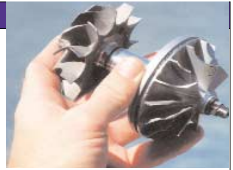
The driving force of the RAJAY turbocharger is the turbine wheel (left) and compressor impeller (right). It is capable of rotating up to 120,000 rpm.
